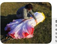
**Step 3.** Group together the middle and the trailing edge (TE) of the wing by sorting the concertina folds near the B and C tabs.
